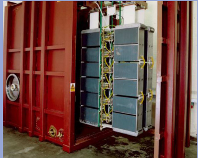
One of the 2.4 megavolt Marx capacitor banks at the Mega Ampere Generator for Plasma Implosion Experiments (MAGPIE), Imperial College London.
